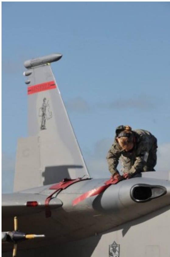
Senior Airman Brittany Dalton, 104th Fighter Wing Crew Chief, installs louver covers on an F-15C Eagle aircraft to prevent foreign objects from accidentally entering the aircraft. Senior Airman Dalton is deployed to Leeuwarden Air Base, Netherlands, with the 131st Expeditionary Fighter Squadron (U.S. Air National Guard photo by Capt. Anthony Mutti)
