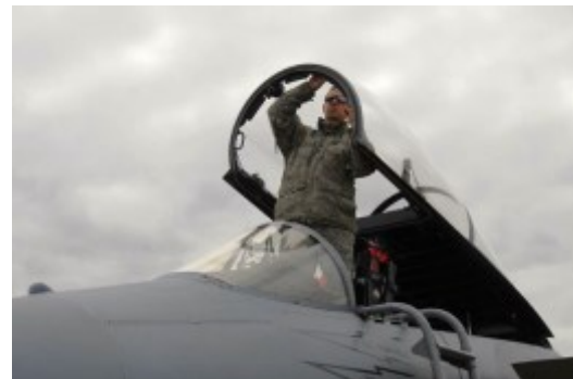
Tech. Sgt. Brian Nason, 104th Aircraft Maintenance Squadron, conducts a visual inspection of the canopy of a F-15C Eagle aircraft (U.S. Air National Guard photo by 1st Lt. Bonnie Harper)
