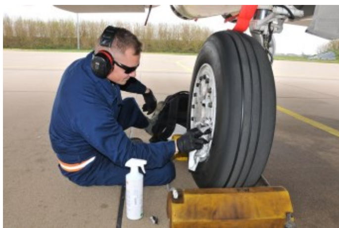
Staff Sgt. Taylor Steadman inspects the wheel of an F-15C Eagle aircraft for cracks and leaks, April 19, 2016, Leeuwarden Air Base, Netherlands. (U.S. Air National Guard photo by Capt. Anthony Mutti)
