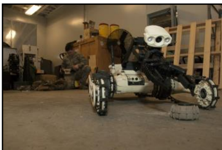
The Micro Tactical Ground Robot used by EOD can fit in a backpack and allows them to safely examine an object. (U.S. Air National Guard Photo by Airman 1st Class Randall S. Burlingame)
